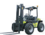
Rough Terrain Forklift
